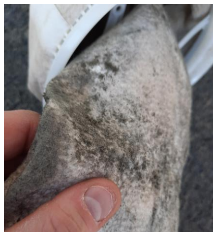
Figure 4: Picture of the sand caught in the ‘bag filters’ of the system during the unloading phase. A limited amount of very fine sands/ silts seem to have been produced.
